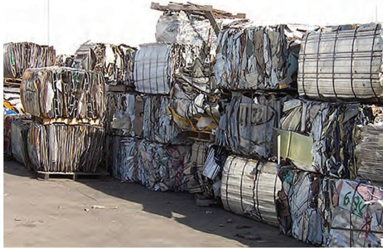
(Above) Bales of steel stacked and ready to be shipped off for recycling. (Below) Scrap metal is collected and crushed into manageable bales to be sent to be recycled. (Right) A trailer load of scrap metal gets dumped off.
